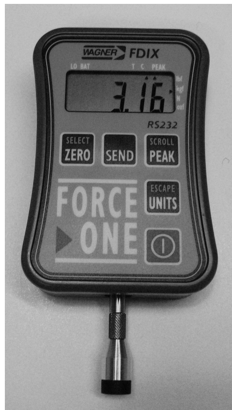
Figure 1. The pressure algometer (Wagner Force One Model FDIX 50TM, Wagner Instruments).
