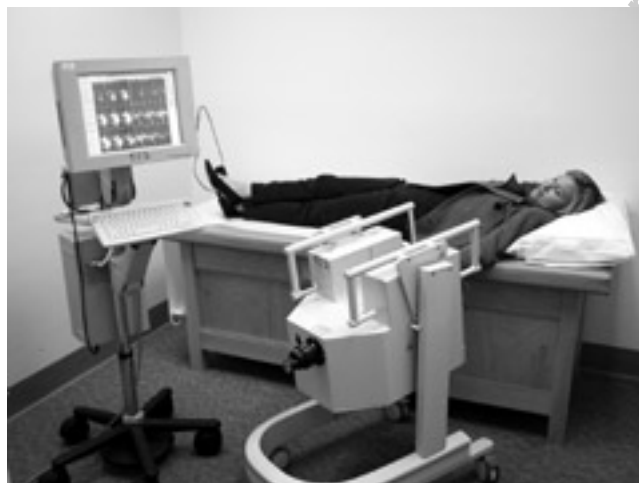
Figure 2. Low-field extremity MRI. A. Lunar (GE/Esaote) 0.2-Tesla extremity MRI system. B. MagneVu 0.2-Tesla portable extremity MRI system.
