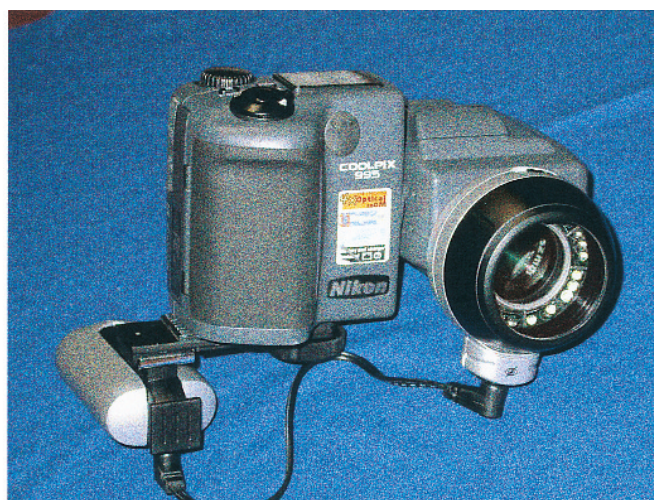
Figure 1. A. DermLite dermoscopy unit. B. DermLite Foto flash-equipped Nikon Coolpix 995 digital camera.
