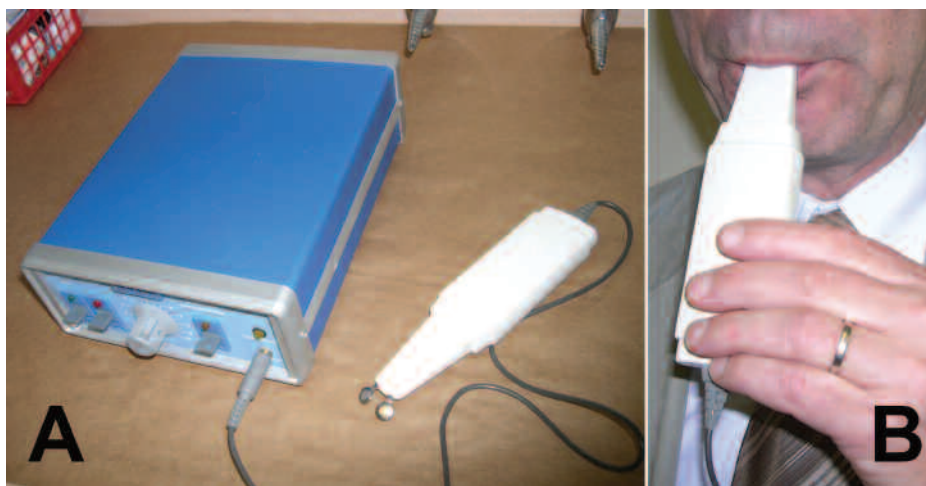
Figure 1. First-generation neuroelectrostimulation device consisted of a hand-held probe, tipped with stainless steel electrodes, and a console that housed a battery and the electronic signal-generating power source, the size and shape of which were similar to a video or CD player.
