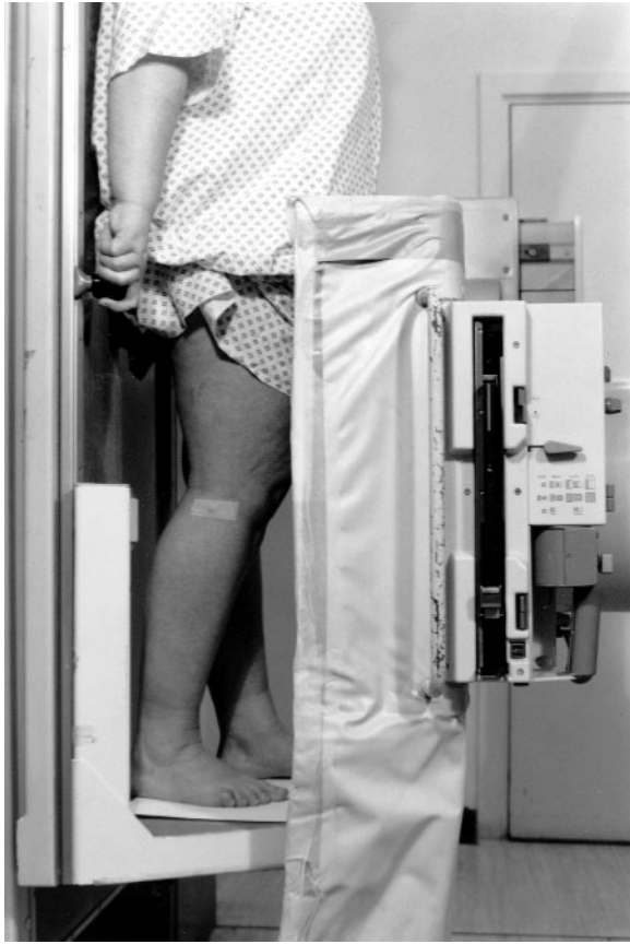
Figure 1. The radiographic examination table tilted vertically, with the fluoroscopic image intensifier and film carrier to the right of the patient standing on a platform. The x-ray tube is located under the examination table.
